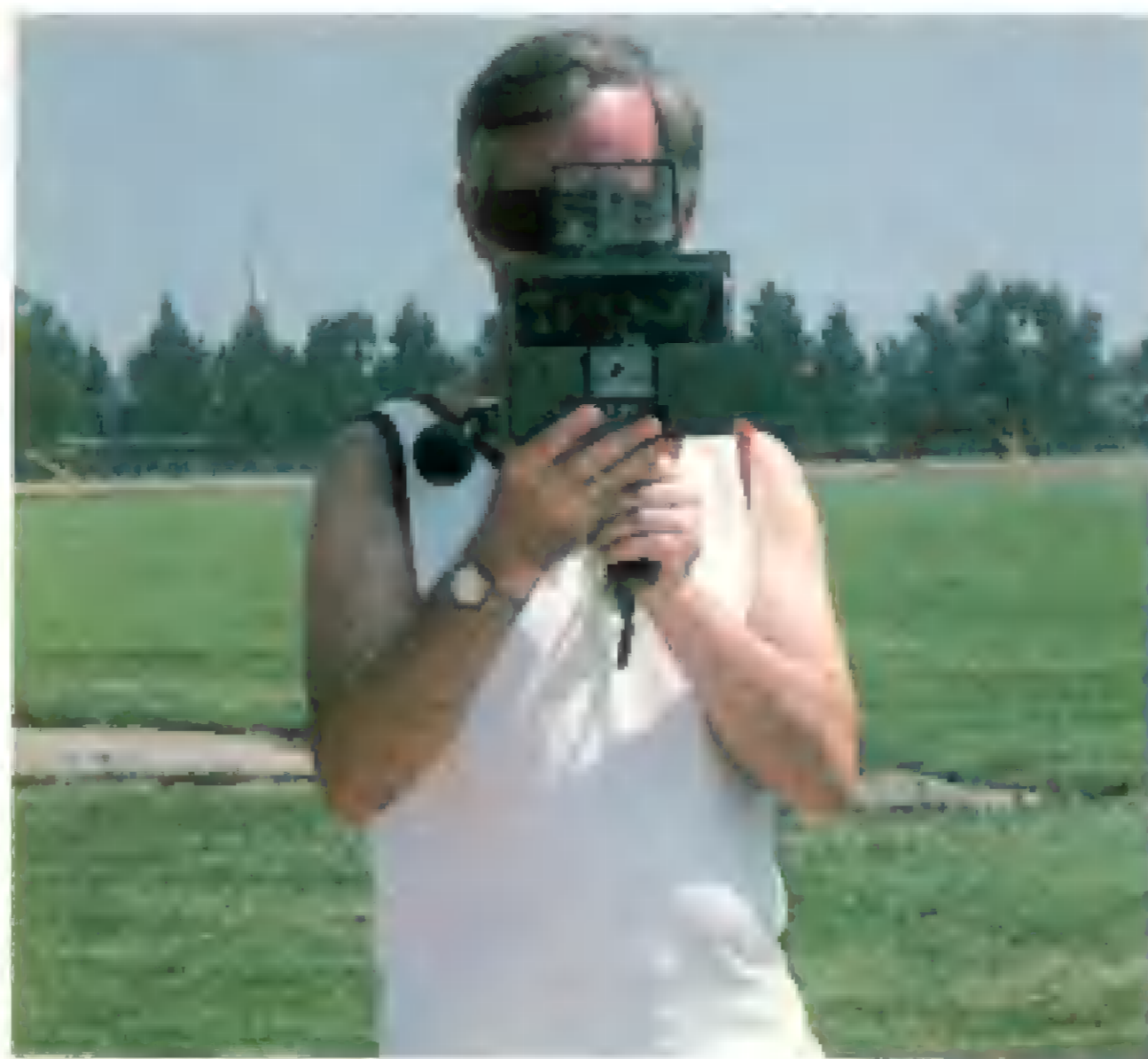
Filmmaker John Hart shoots Super-8 3-D with a custom designed mirror box attachment. Image format is the same as with the Elmo 3-D attachment.
